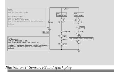
In the first pic, there's a schematic of a basic current mirror configuration that is built of two 300V PNP small signal transistors (BF421 because they were the nicest ones easily available). Then there's the good old diode (huge voltage rating, so it's actually a chain of 1000V controlled avalanche ones in a 5mm silicone tube), and a current source to simulate the ion current.
